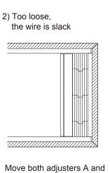
B in the tightening direction
